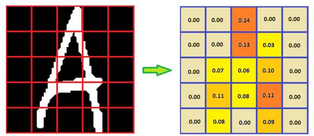
Figure 30. 2D Histogram feature example for the letter A.
